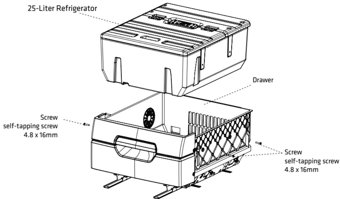
**Note 1:** The screws should be fixed with low torque, because the refrigerator fits perfectly in the truck's original drawer. The fixing of the screws serves for a better adjustment between drawer and refrigerator, eliminating possible gaps.
