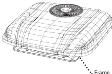
The air inlet is behind and under the appliance. Clean underneath, between the ceiling and the base of the appliance. Space is restricted (minimum 25mm).
