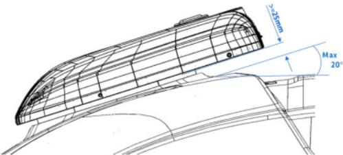
**10.1** There must be a minimum distance of 25mm between the base of the AC and the surface of the ceiling so that air can enter the condenser without losing flow.
